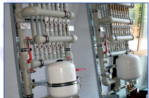
Fabrication of storey stations and distributors according to plan
